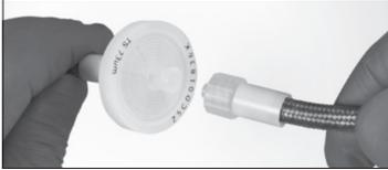
3. Remove the old filter disk by holding it in one hand and loosening it by twisting it off the hose connectors on either side. They rotate in opposite directions.
